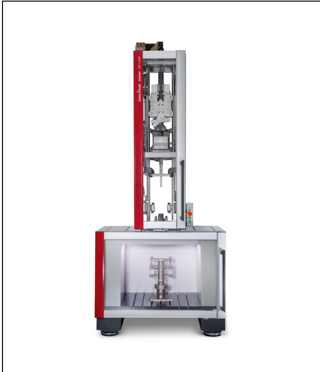
Amsler HIT1100F, multiaxial impact test
