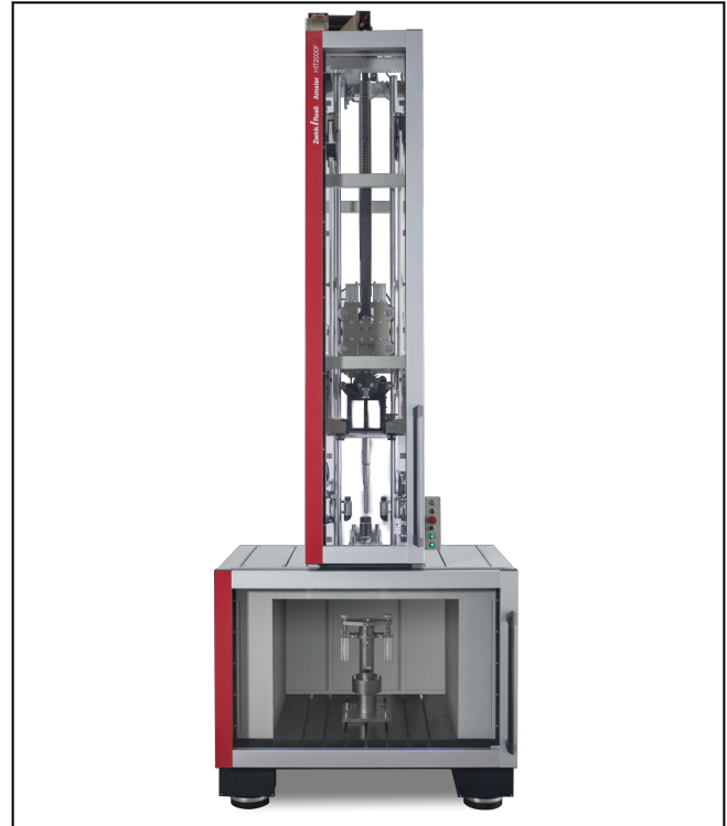
Amsler HIT2000F, multiaxial impact test
