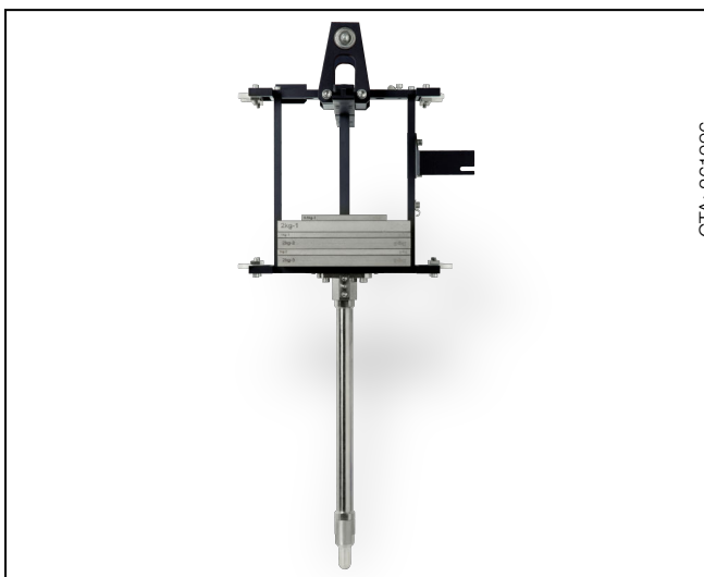
Mass carriage with single masses and Impactor
