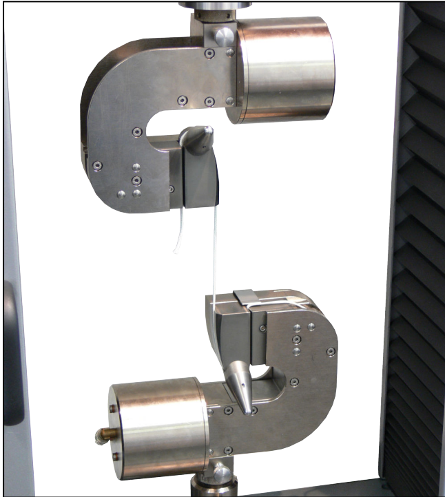
Capstan grips for high-strength plastic yarns type 8297, Fmax 2.5 kN
